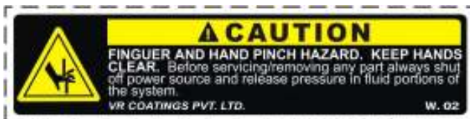
Label on pump provided without coupling guard.
