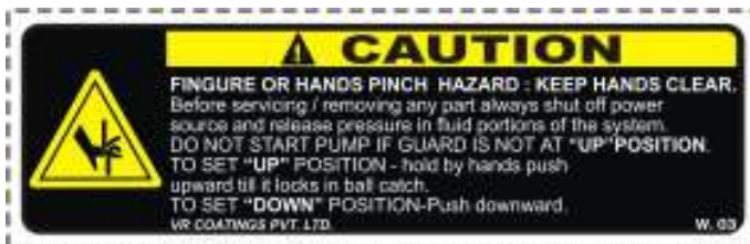
Label on pump provided with coupling guard.
